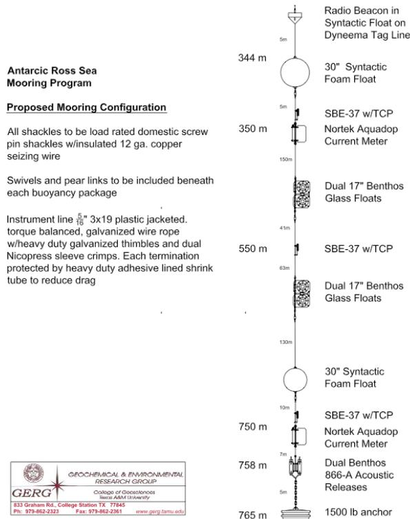
**Figure 1:** Schematic of mooring design.
