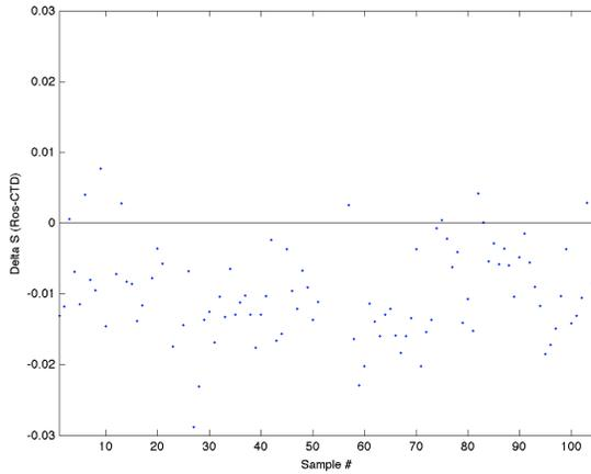
**Figure 2:** Salinity difference, DeltaS (Rosette-CTD), vs. Sample number for conductivity sensor.
